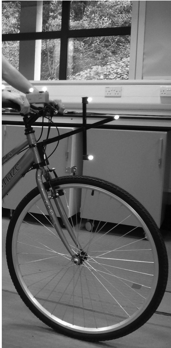
Figure 3.1 Bicycle setup with all the markers. Two markers were positioned on the stem and three on the T-frame.
