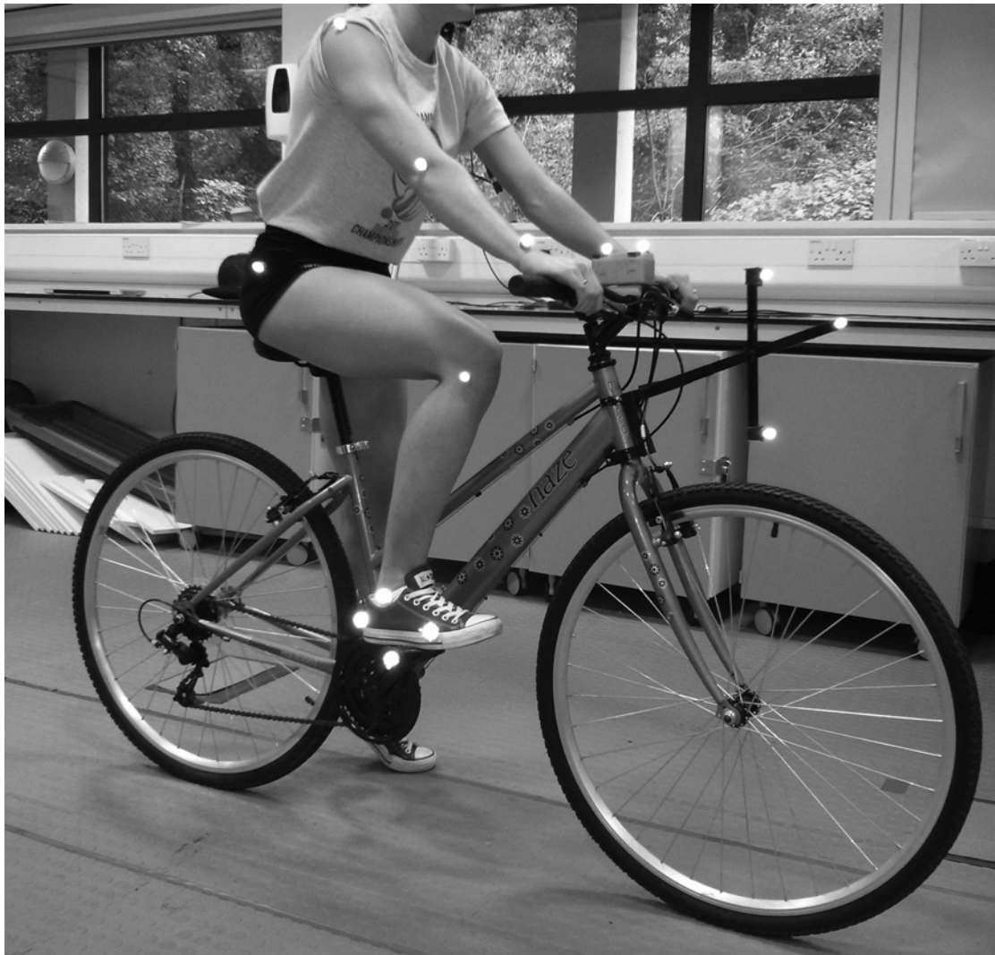
Figure 4.1: Bicycle and participant setup. Reflective markers were put on the main anatomical points of the body and on the bicycle with a custom designed T-frame in front allowing us to calculate steering and leaning parameters.
