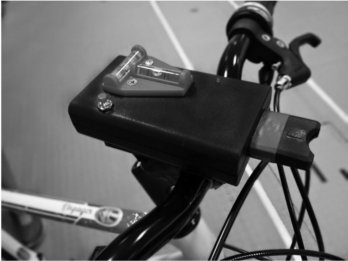
Figure 2.8: Box with a data logger and sensor to record steering and roll rate. On the surface there are two spirit levels for the initial setup to make the device as level as possible, a button to start and stop the recordings and an LED light indication, which is switched on during the recordings.
