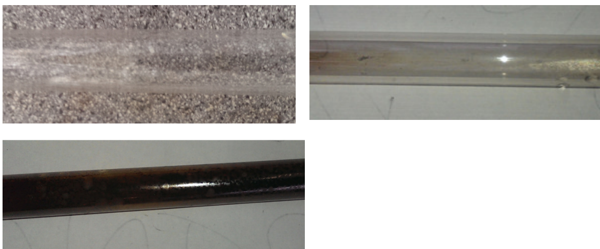
Figure 5.11: Comparison of tar fouling the sample holder; (left to right) clean sample holder - sample holder after RSB gasification and sample holder after WPB gasification. Experiments were carried out 850°C using a steam flow rate of 172 \text{ g min}^{-1} \text{ kg}^{-1} biochar
