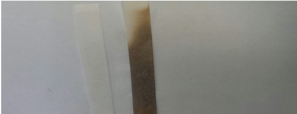
Figure 7.2: Results of the lead acetate test confirming the presence of H_2S , (left) N_2 , (right) RSB syngas
