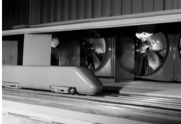
Figure 23 ICE2 model and crosswind generator used in (Baker et al., 2001)
