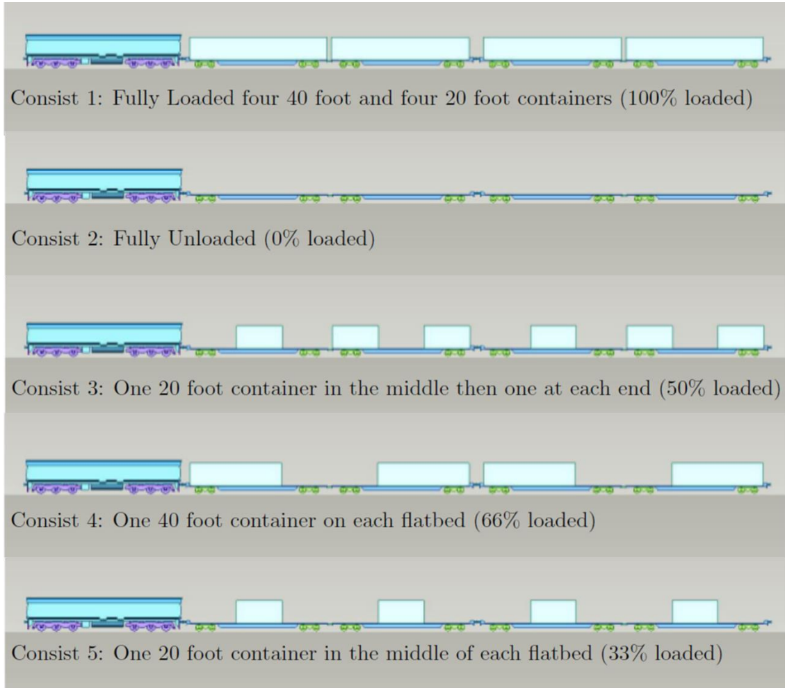
Figure 9 Loading configurations used by Soper (2014)
