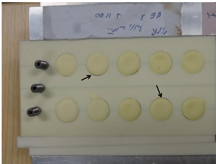
Figure 3.15: Example of specimens of 20% emulsion after 24h at 20 °C. The arrows indicated portions where sample contraction is well visible.
