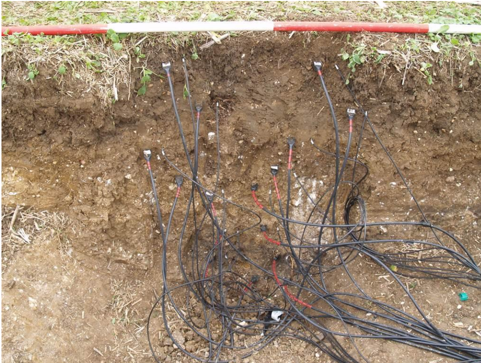
Figure 3.21: The inserted probes at DCFA in the ditch section
