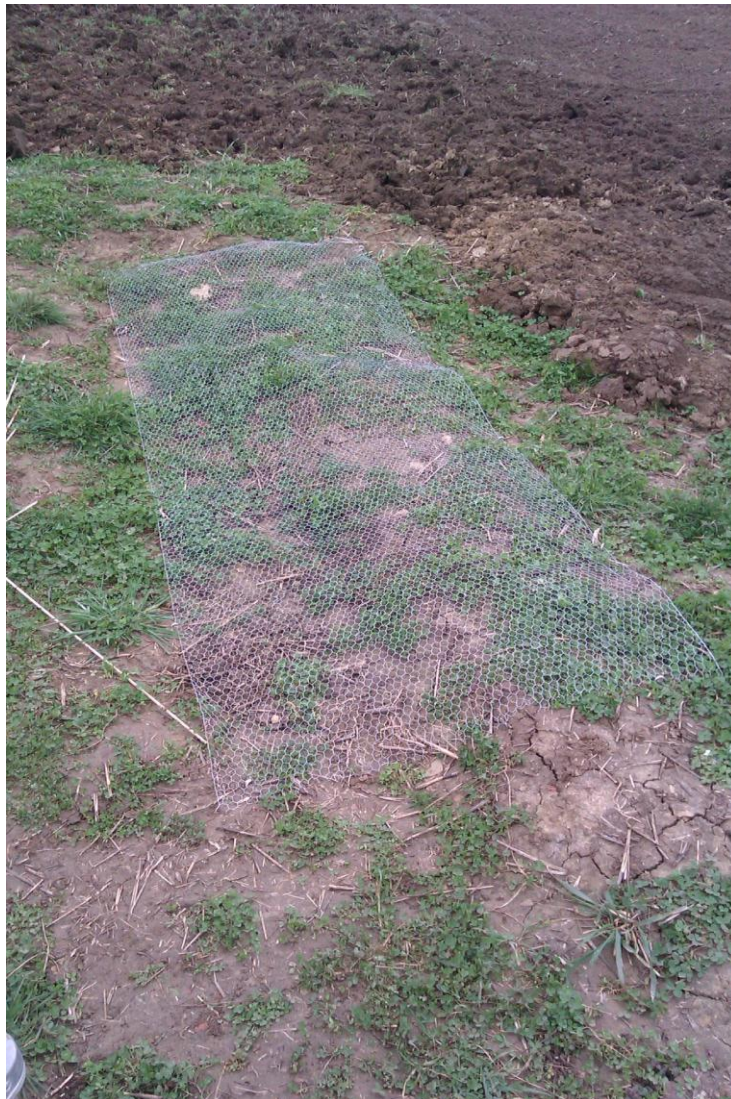
Figure 3.31: Wire mesh used to protect the probe locations from burrowing wildlife
