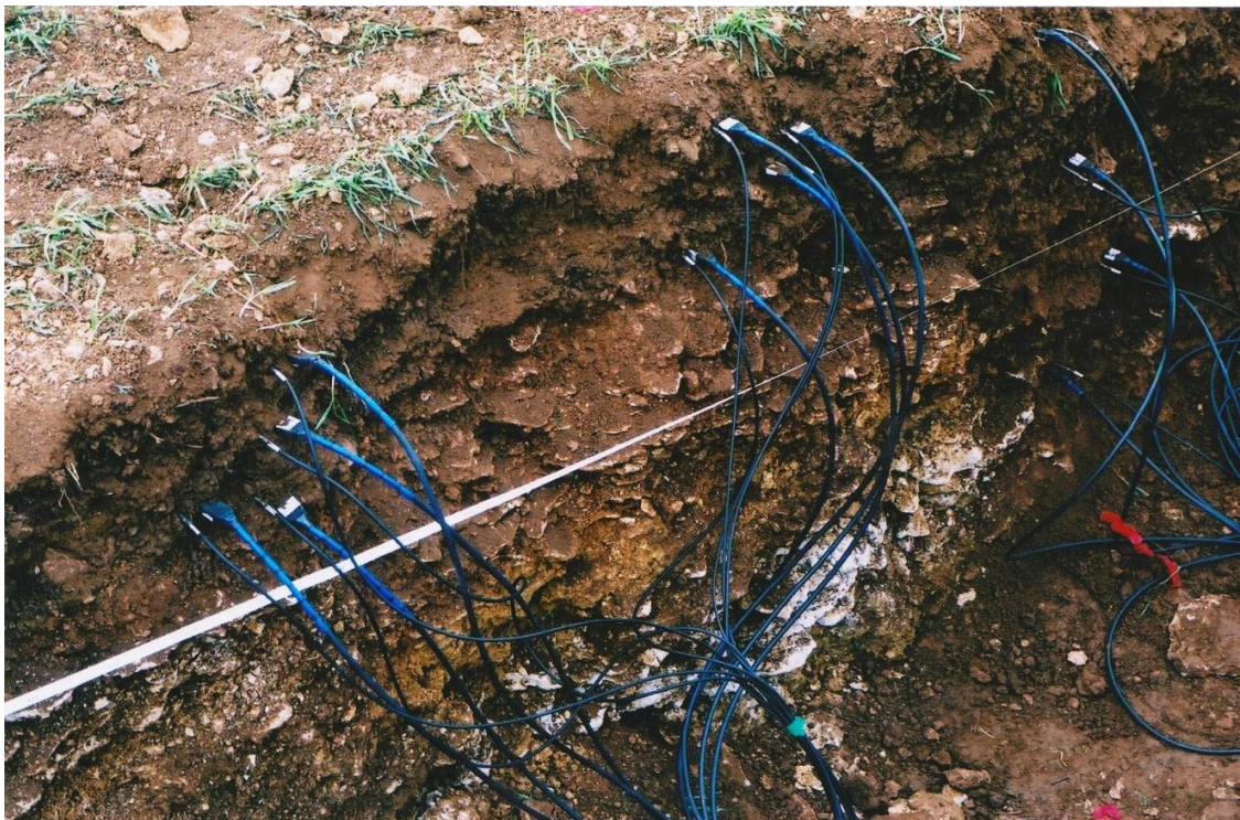
Figure 3.24: The inserted probes at CCC in the SSM. Note the rock below c. 0.2m depth
