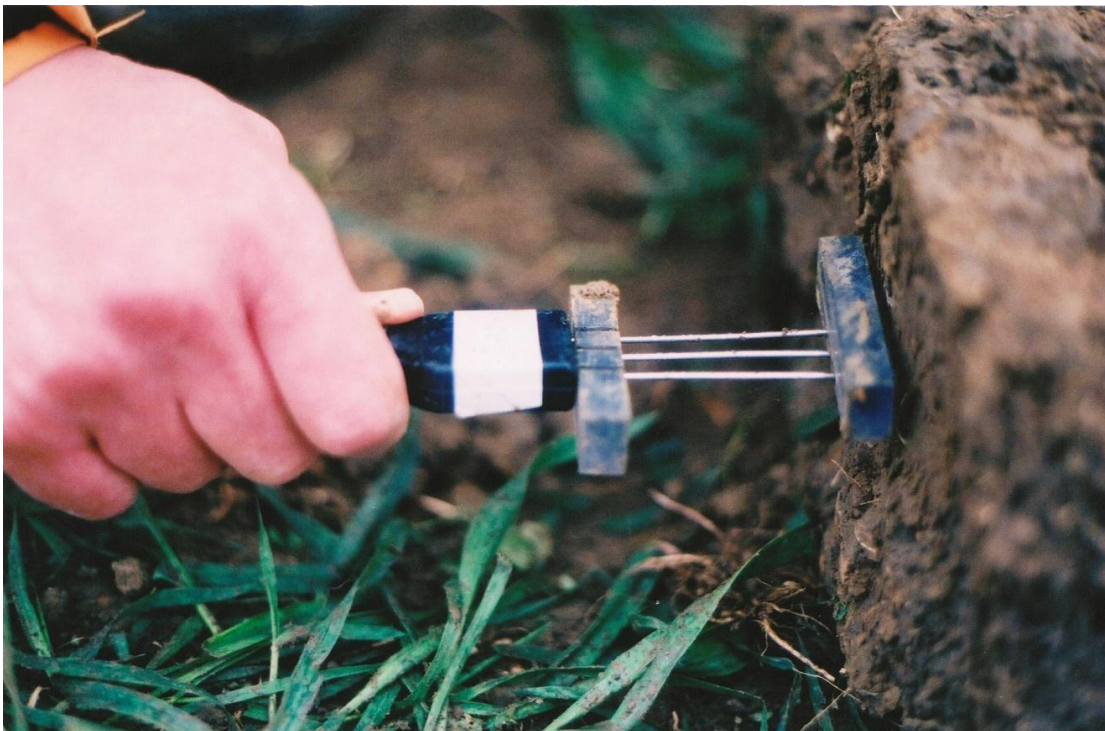
Figure 3.20: The insertion of the TDR probes using plastic waveguides to keep rods parallel
