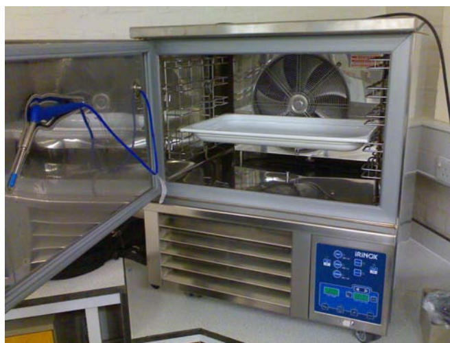
Figure 39 – Blast freezer used for rapid laboratory freezing (Irinox, Italy)
