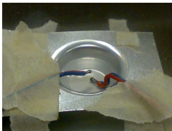
Figure 41 – The preparation of a blister with thermocouples prior to temperature measurement.
