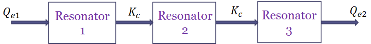
Figure A9 The block diagram of the third order resonator filter to be designed- drawn by the student
