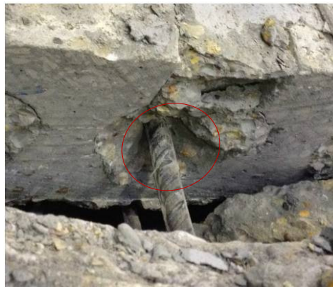
Figure 3.44 Cone failure around the middle bar (taken near 1MR in FT3) at deflection of 347mm
