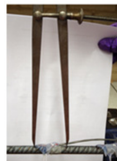
Figure 3.21 Marked points on the bar at the middle joint to measure permanent elongation
