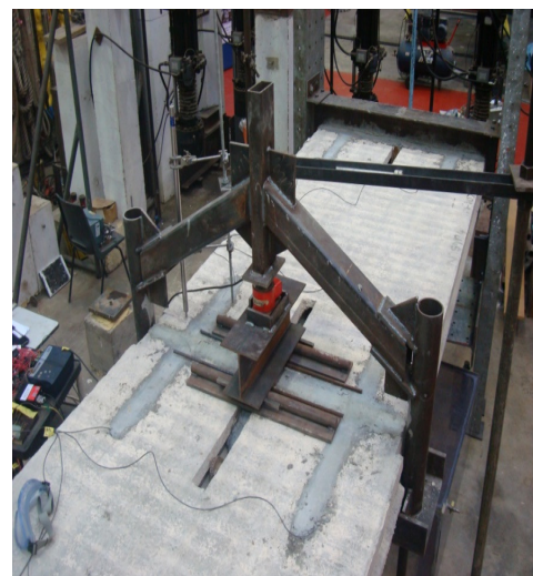
Fig. 3B. 3 Elevation of loading details at floor-to-floor joint
