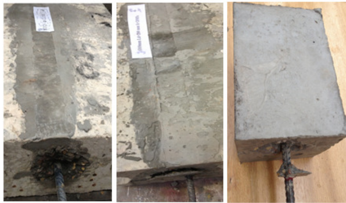
Figure 3.13 Cone failure at the loaded end of precast and prism specimens - pullout failure mode
