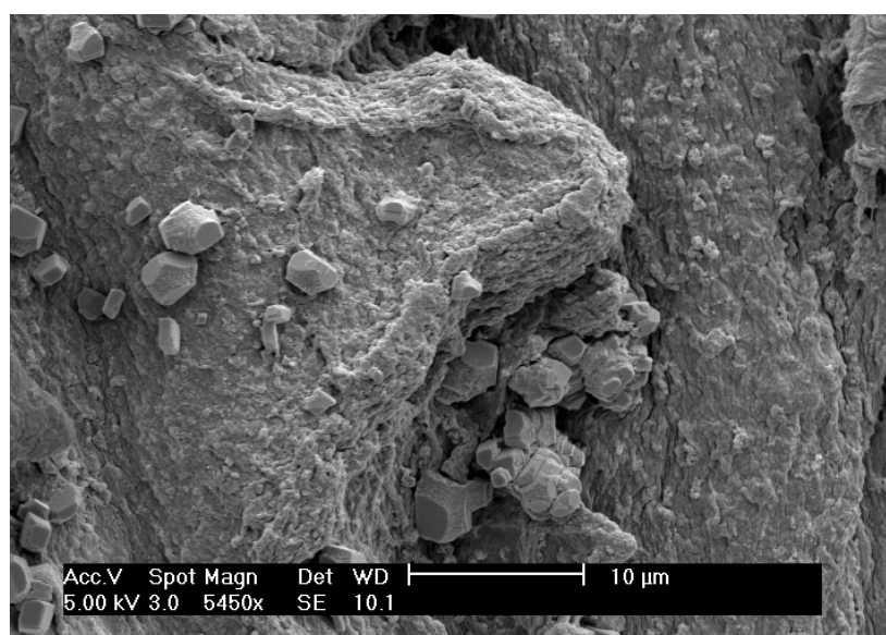
Fig. 33. ESEM image of bacterial cellulose hydrolysed by 15% NaOH (30mins)
