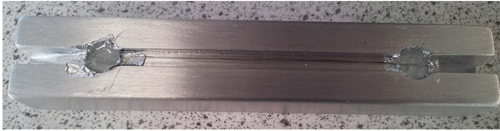
Figure 30: Bespoke carbon fibre alignment tool, manufactured by University of Birmingham, showing aligned fibre bundle set in Araldite Rapid resin
