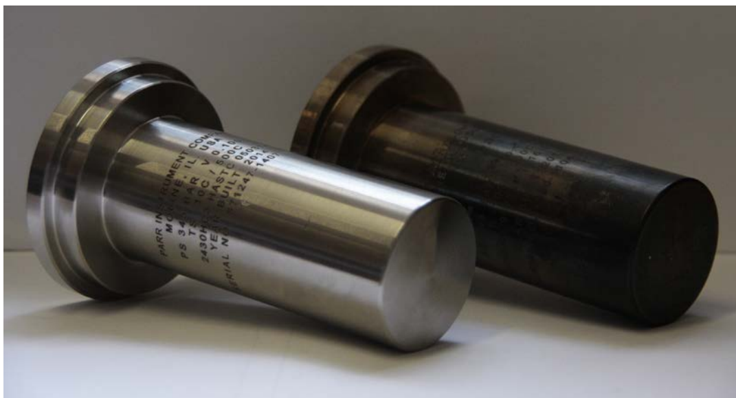
Figure 6: High-Temperature Reactors showing the discolouration at the end-of-life of the reactor, Hastelloy (left), stainless-steel (right)
