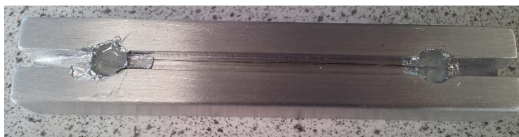
Figure 8: Bespoke carbon fibre alignment tool, stainless steel, approximately 120 mm in length
