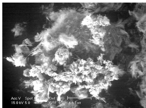
Figure 3.3.12.6: ESEM Image of Alkyl Phosphate Modified Calcium Pyrophosphate Showing Fibrous Morphology.
