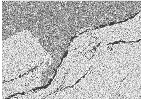
Figure 4: Image showing grain boundary between a region of quartz and a region of K-feldspar in a granite (Eberhardt et al 1999)
