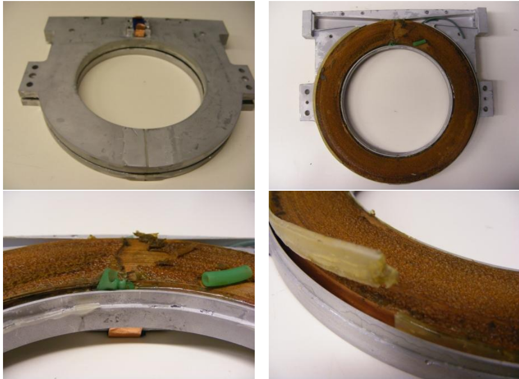
Figure A.1: Opening of the old moving coils. (Top left) the coil with all the external glue removed, (top right) view of the internal body after opening, (bottom left) close-up of the damage to the rubber, and (bottom right) displaced brittle glue inside the cooling body.
