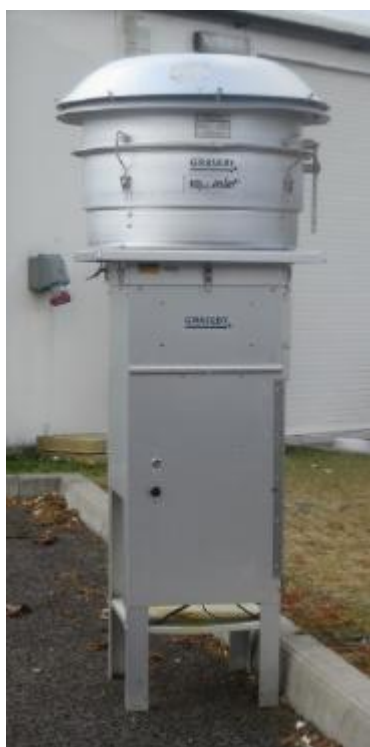
Figure 2.2. Pictures of samplers used at UK PAH monitoring sites (Brown et al., 2011).
