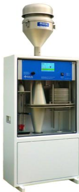
Figure 2.2. Pictures of samplers used at UK PAH monitoring sites (Brown et al., 2011).
