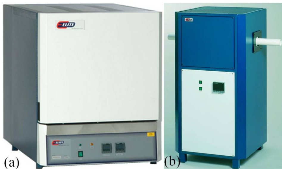
Figure 2.38. Images of conventional furnaces. (a) is box furnace and (b) is tube furnace.
