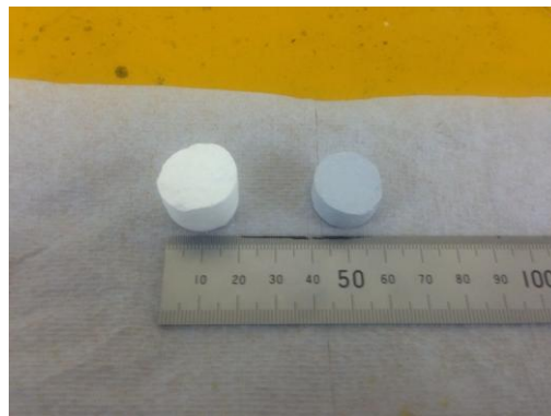
Figure 5.3. An image of the typical green compacts formed by CIP. White is the pure \text{Al}_2\text{O}_3 and blue is the GPL/ \text{Al}_2\text{O}_3 sample.
