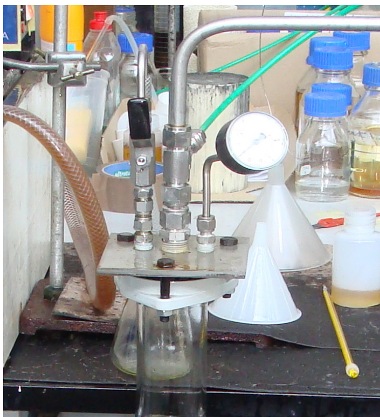
Figure 6-2. The top part inlet of the DGCR rig.
