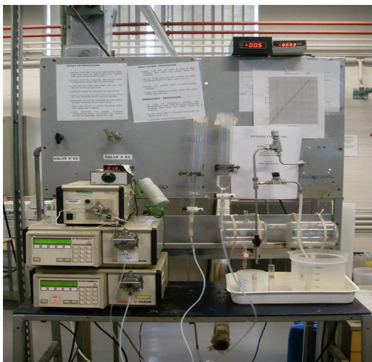
Figure 3-4. Image showing the two HPLC pumps, a static mixer and feeding columns.
