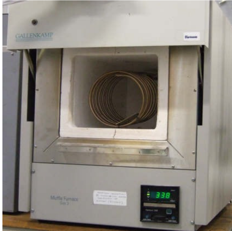
Figure 3-5. Image of tubular coil reactor housed in the electrical furnace.
