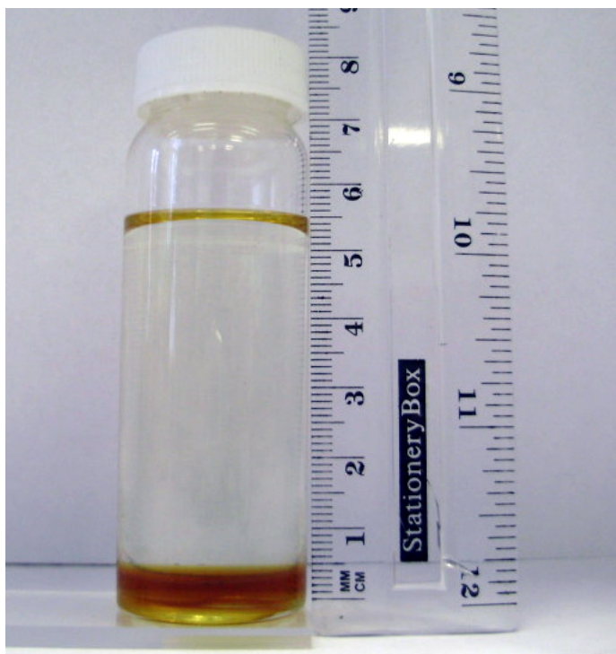
Figure 6-9. Sample product of biodiesel from DGCR rig. The upper layer is biodiesel and the lower layer is residual catalyst with glycerol.
