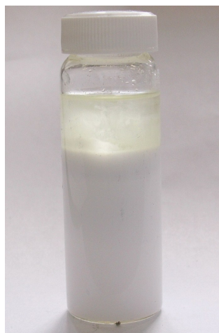
Figure 3-6. Sample of hydrolyzed sunflower oil: upper layer (FFA, TG,DG and MG) and lower layer (G and water).
