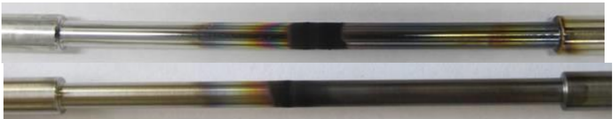
Figure 6.8 HLPS Tubes after a testing using SPC 2 at 350°C, Electropolished (Top) and Standard (Bottom)
