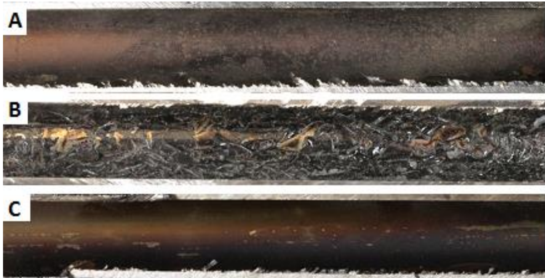
Figure 5.23 Feed Pipe Simulator deposit images under a range of shutdown conditions (a) continuous oil flowing (b) drained shutdown (c) flooded shutdown
