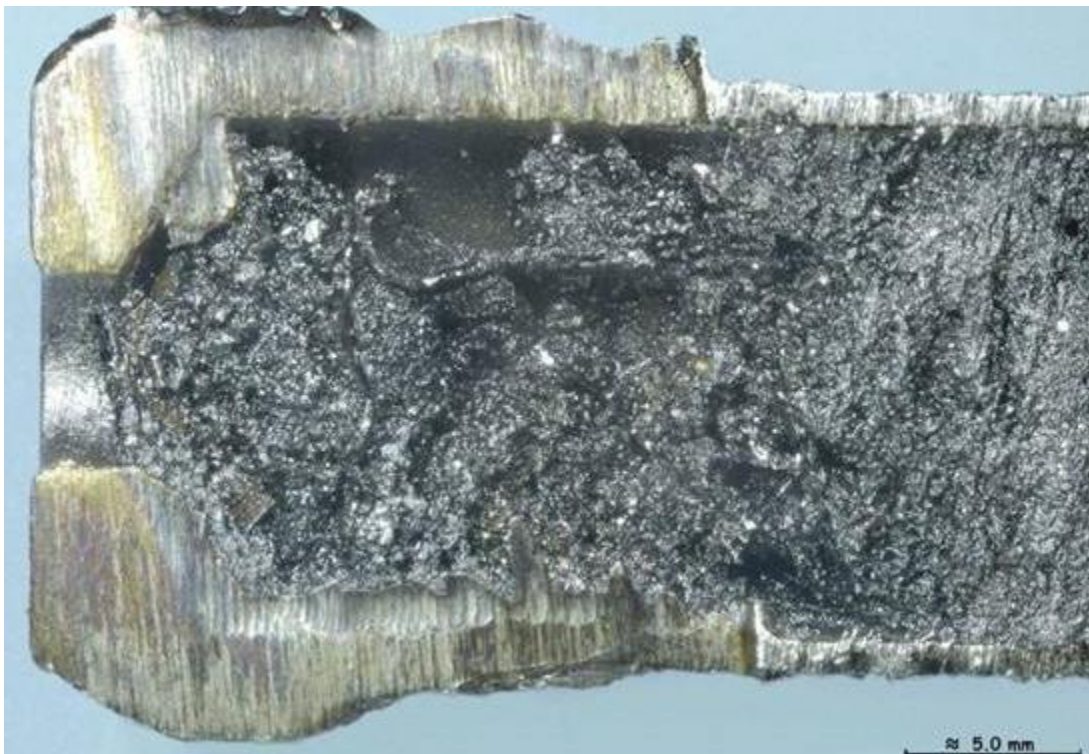
Figure 5.15 An example of gas turbine vent pipe deposits
