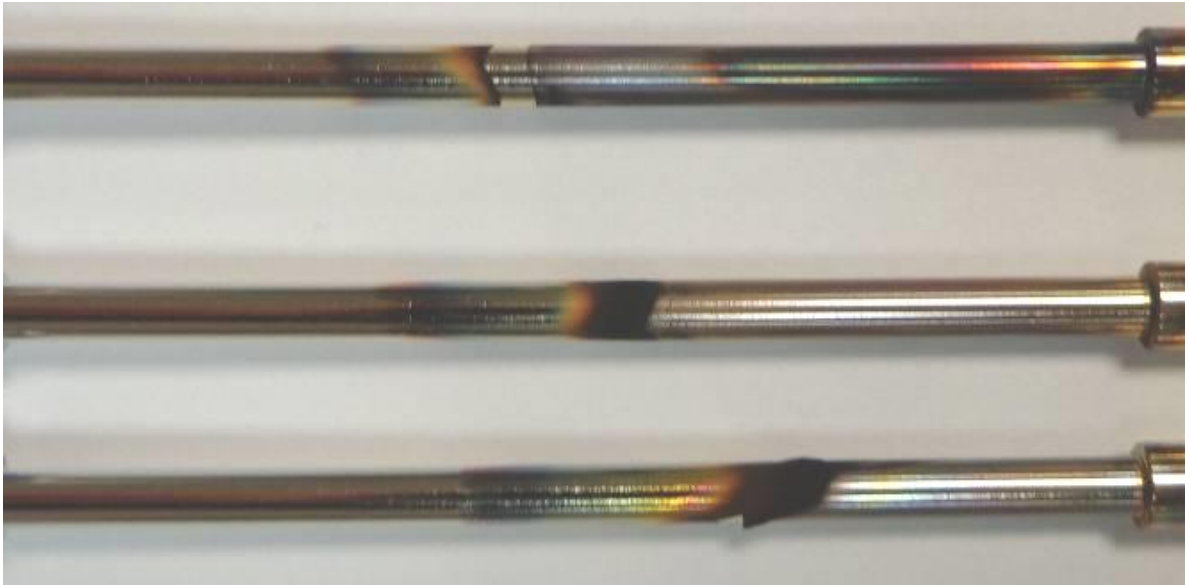
Figure 6.10 Image showing deposit on SPC 1 electropolished test specimens at 375 °C (Top), 350 °C (Middle), and 325 °C (Bottom)
