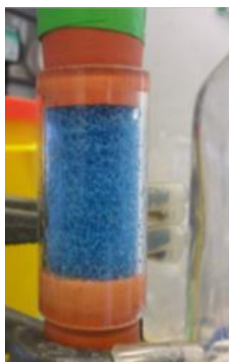
Figure 7: Column packed with 8 foam discs.
