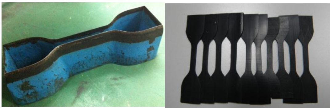
(a) The cutters (b) The dumb-bell shaped test pieces
