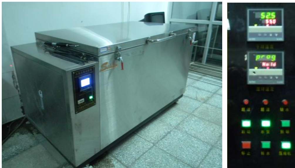
(a). High temperature and RH cycling test chamber (b). Control panel
