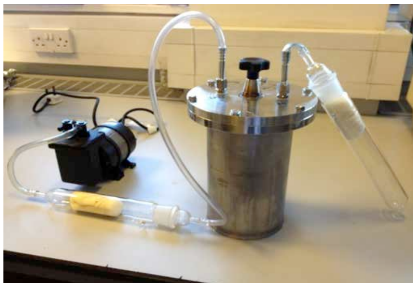
Figure 2.1: UoB chamber configuration showing the stainless steel test chamber with connected air pump and collection PUFs
