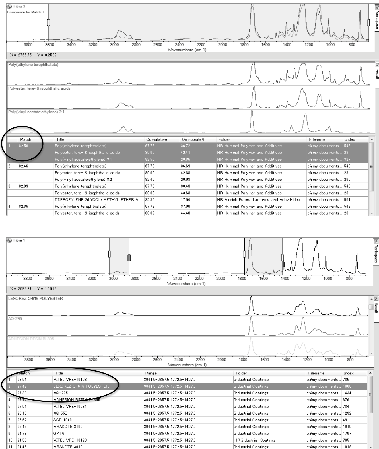
Figure 5.8: Returned database spectral searches of (Top) entire sample spectrum showing an 83% match with polyester and other industrial coatings, (Middle) highlighted peaks of interest showing a 97% match with polyester and (Overleaf) comparison of the fibre, polyester reference and HBCD reference spectra
