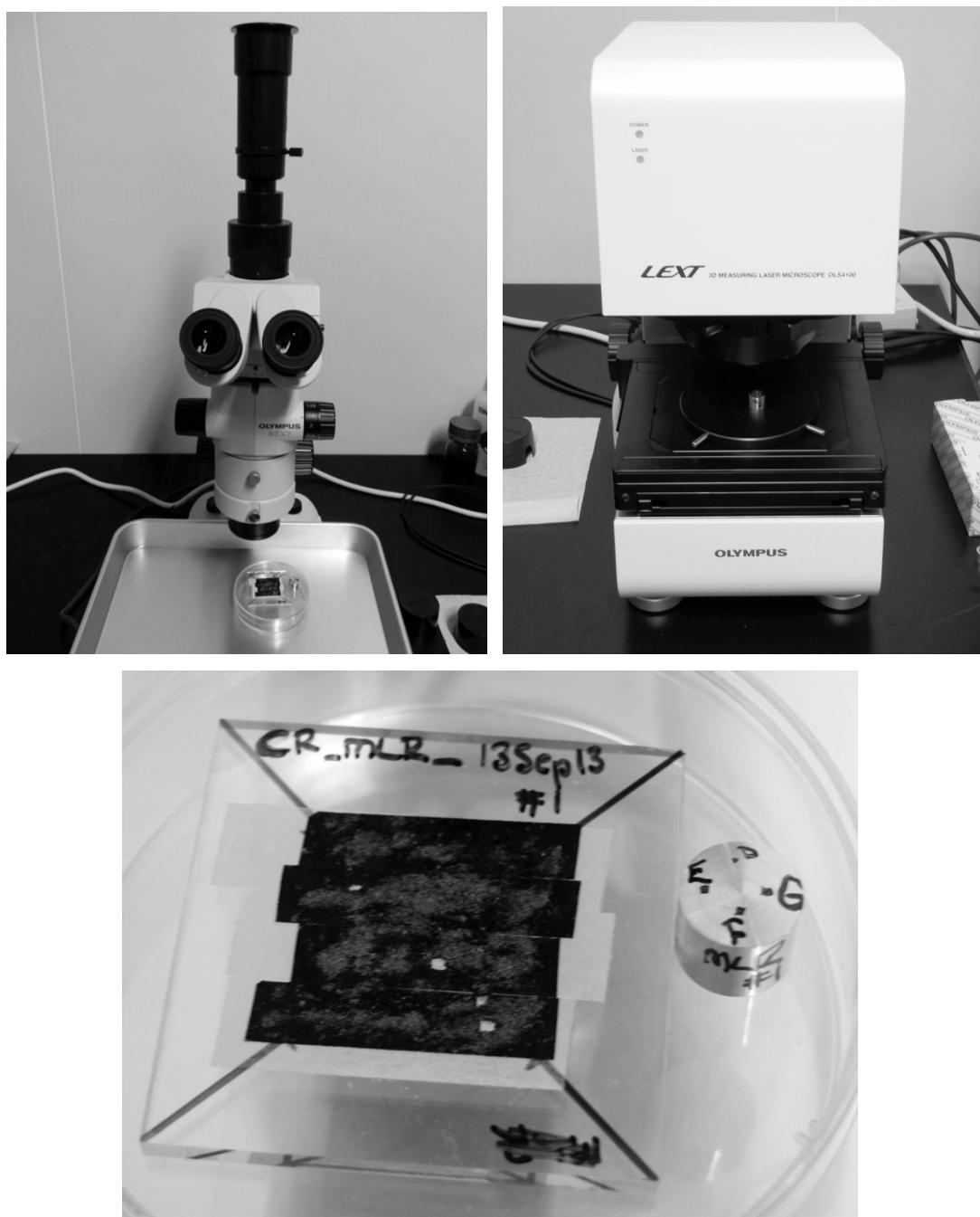
Figure 5.11: Pictures of (Left) microscope used for removing 2 x 2 mm areas of interest from sample to aluminium stub (Right) LEXT 3D laser microscope with sample stub (Bottom) 25 x 25 mm sample with removed region placed on stub
