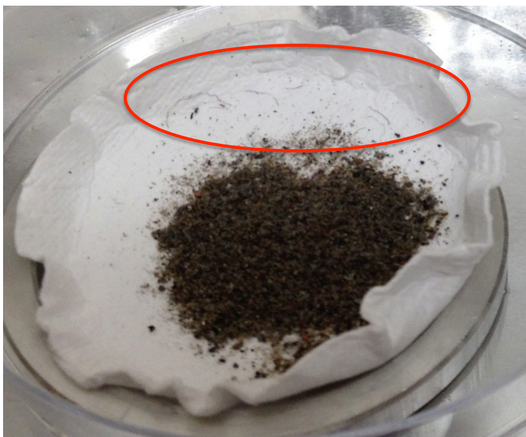
Figure 3.12: Image of a chamber dust sample post volatilisation experiment with HBCD treated curtains in the Micro chamber. Visible fibres present in the dust sample are circled.
