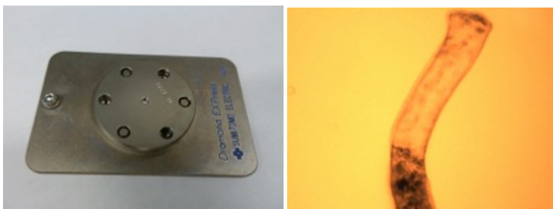
Figure 5.7: Diamond compression cell used for %Transmission FTIR analysis and captured image of the collected fibre ‘squashed’ in the cell
