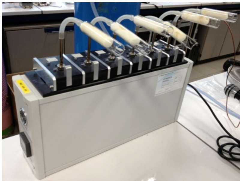
Figure 2.2: Photograph of micro chamber configuration, showing 6 linked chambers
