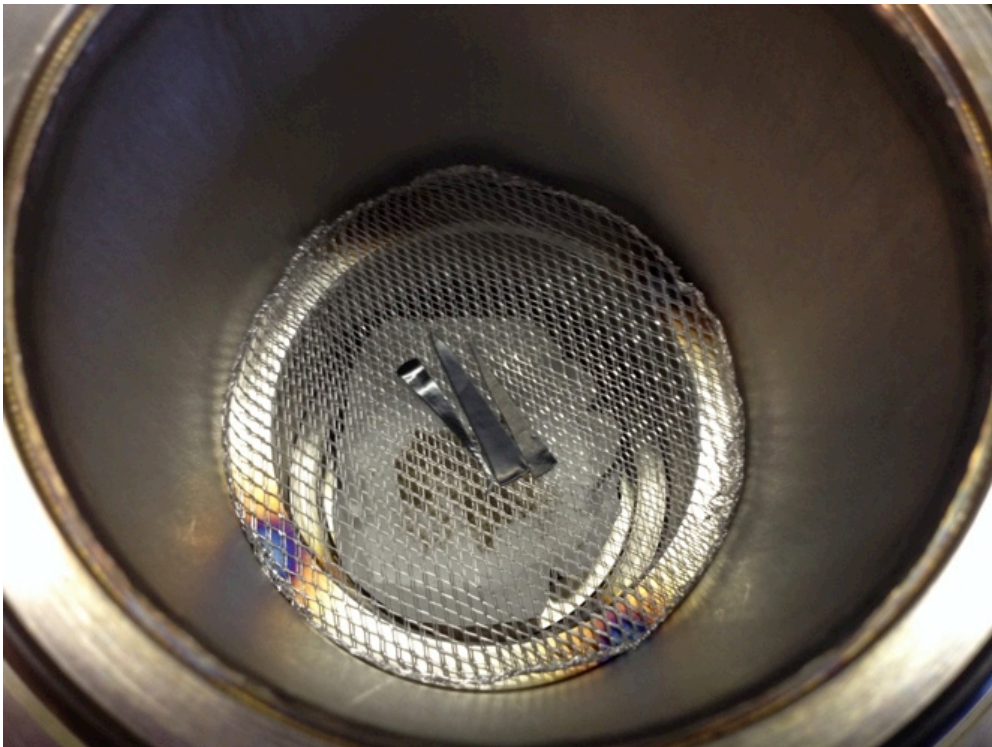
Figure 6.1: Internal test chamber experiment configuration for investigating migration of PBDEs from TV casing to dust via volatilisation and deposition to dust
