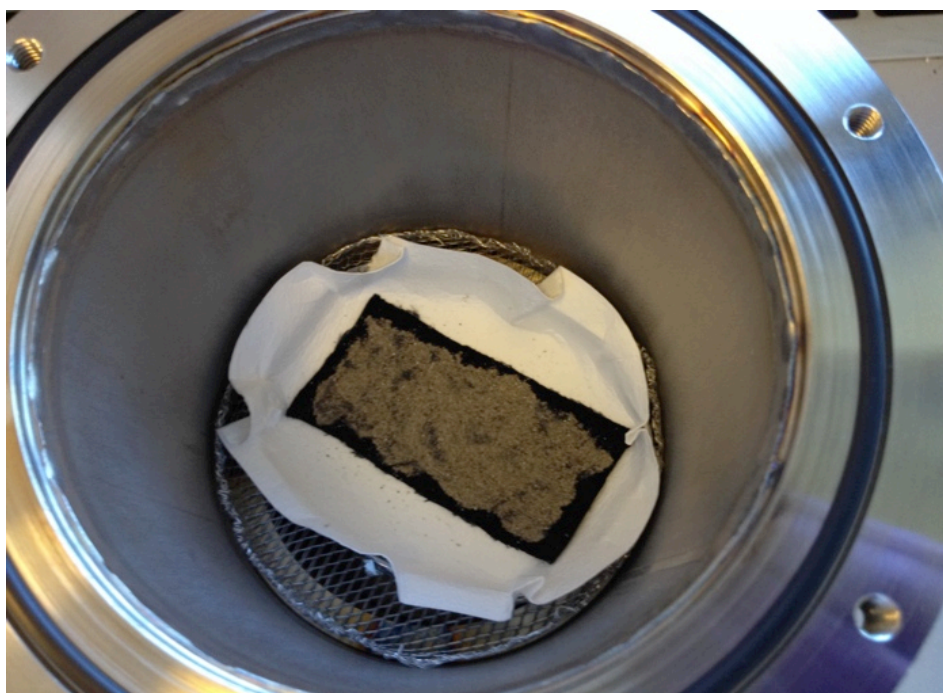
Figure 4.3: Chamber experimental configuration for studying direct contact of HBCDs from a treated curtain to dust
