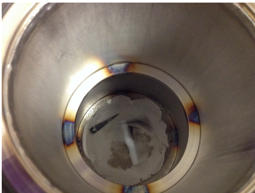
Figure 6.2: Internal test chamber configuration for investigating migration of PBDEs from plastic to dust via abrasion of fine particles
