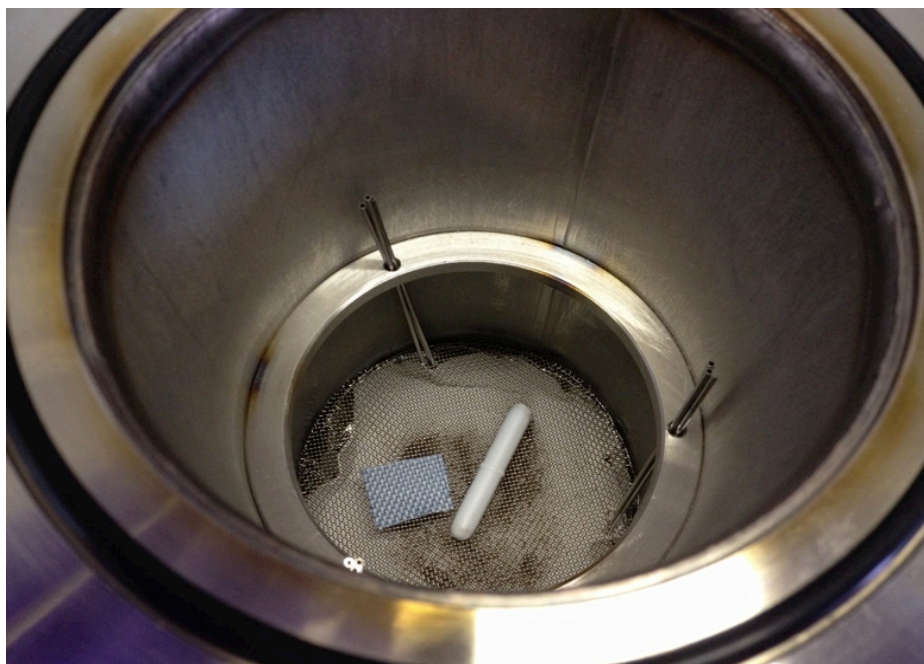
Figure 4.1: Experimental configuration for chamber experiments evaluating abrasion of HBCD treated curtains
