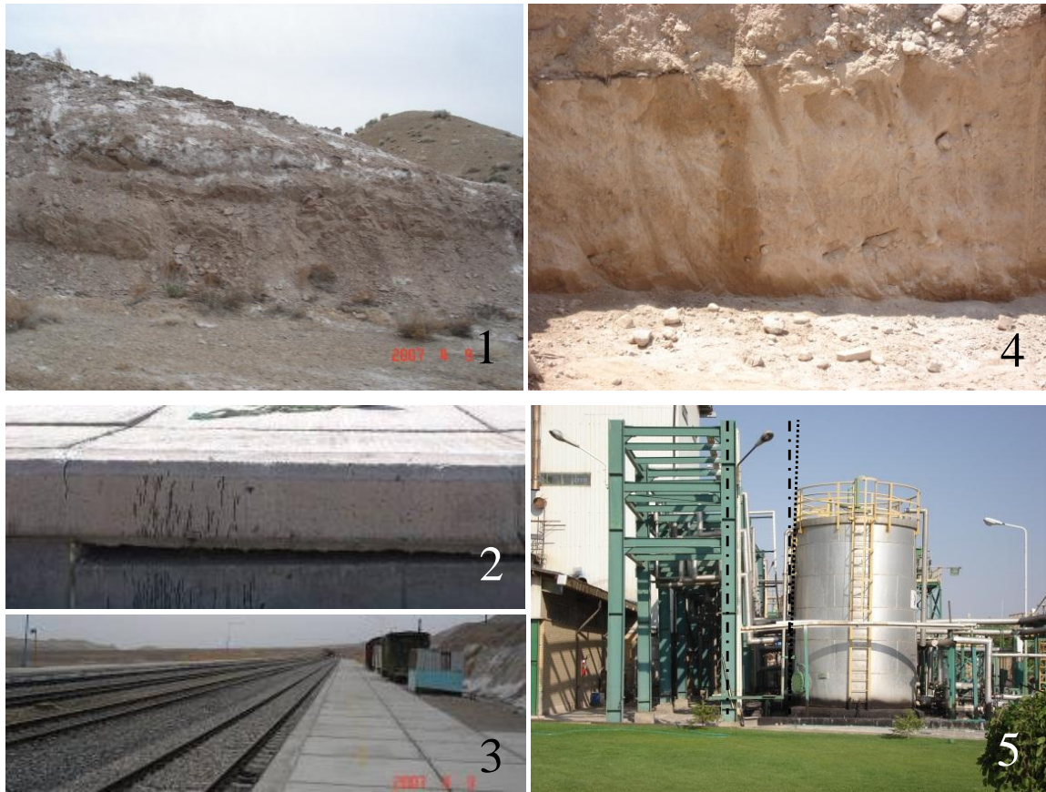
Plate 1.2 [1-2-3] Collapse of calcareous chalky silt soil (containing 10.8% chalk \text{CaSO}_4 \cdot 2\text{H}_2\text{O} , 5.4% \text{SO}_3^{2-} at the pH of 9.3 and calcite contents) beneath a rail-track (Assadi, 2007), [4-5] collapse in a chemical plant after dissolution of secondary crystals of Sodium Hydroxide connectors upon ingress of rain water (Assadi, 2009)
