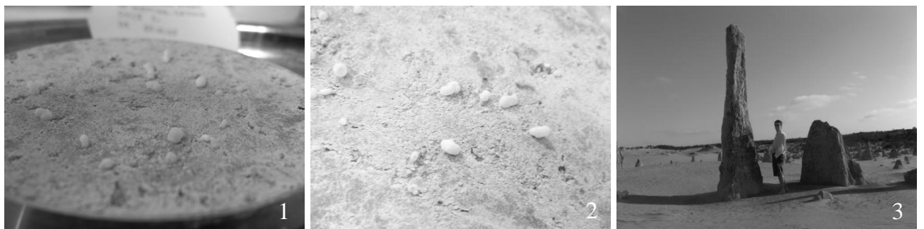
Plate 3.3 Natural lithification of Calcium Carbonate: [1] and [2] Lab-scale synthesis; [3] Combination of dissolution-re-precipitation of Calcium Carbonate close to plant roots at Nambung National Park, Australia (Van Paassen, 2009)
