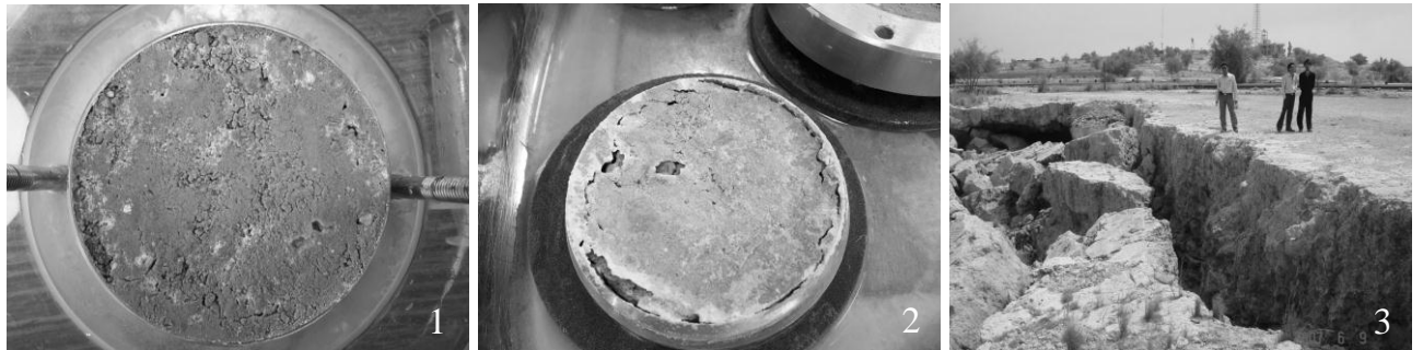
Plate 3.2 [1], [2]: First and second wetting phases along the chemical treatment, [3] Kharg Island, the Gulf: the biogenic Calcium Carbonate (coral reef) and the underlying ML calcareous sand (Nasrollahi and Assadi, 2007, Van Paassen, 2009) which was mirrored in engineered specimens as a chloride-carbonate fragile skeleton
