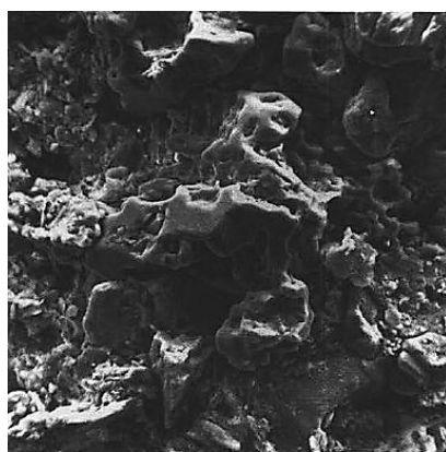
Fig. 2.4 Carbonate connectors under the ESEM microscope
