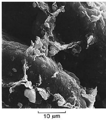
Fig. 2.3 Clay connectors under the ESEM microscope (a) Bridge in UK loess from Kent, in Derbyshire and Mellors (1988)
