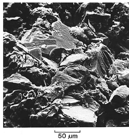
Fig. 2.5 Smooth precipitated silica in palaeosol 10 , Lanzhou, China in Derbyshire and Mellors (1988)
