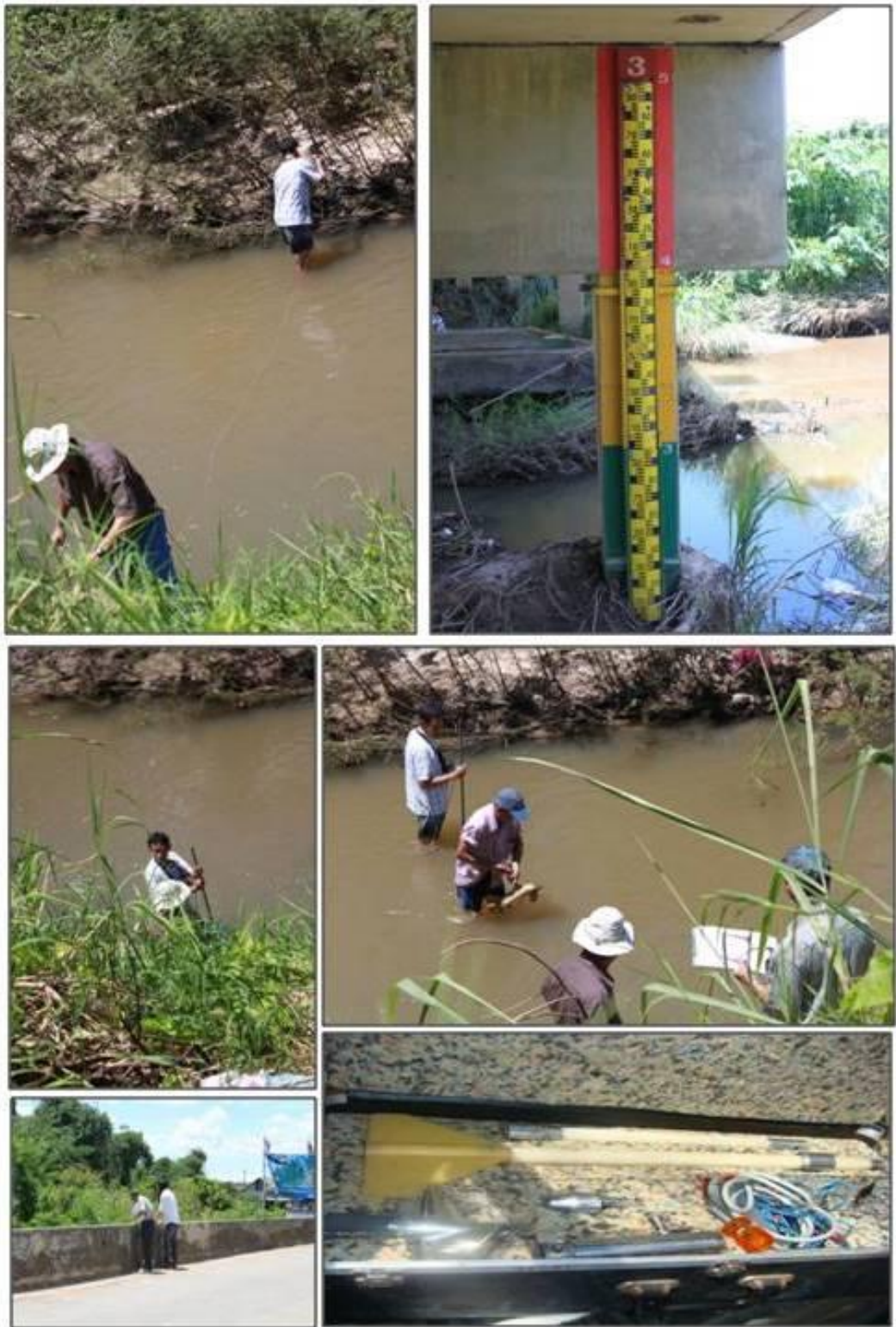
Figure IV-3: Suspended sediment collection demonstrated by RID's staffs at station P21 (Mae Rim River, Mae Rim watershed, NW Thailand)
