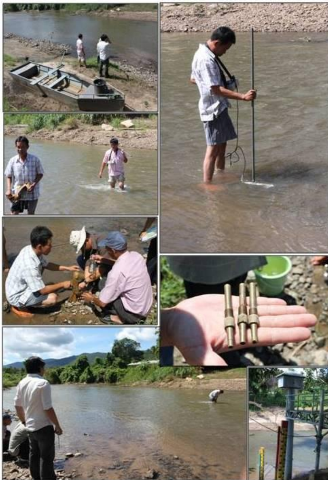
Figure IV-4: Suspended sediment collection demonstrated by RID's staffs at station P84
