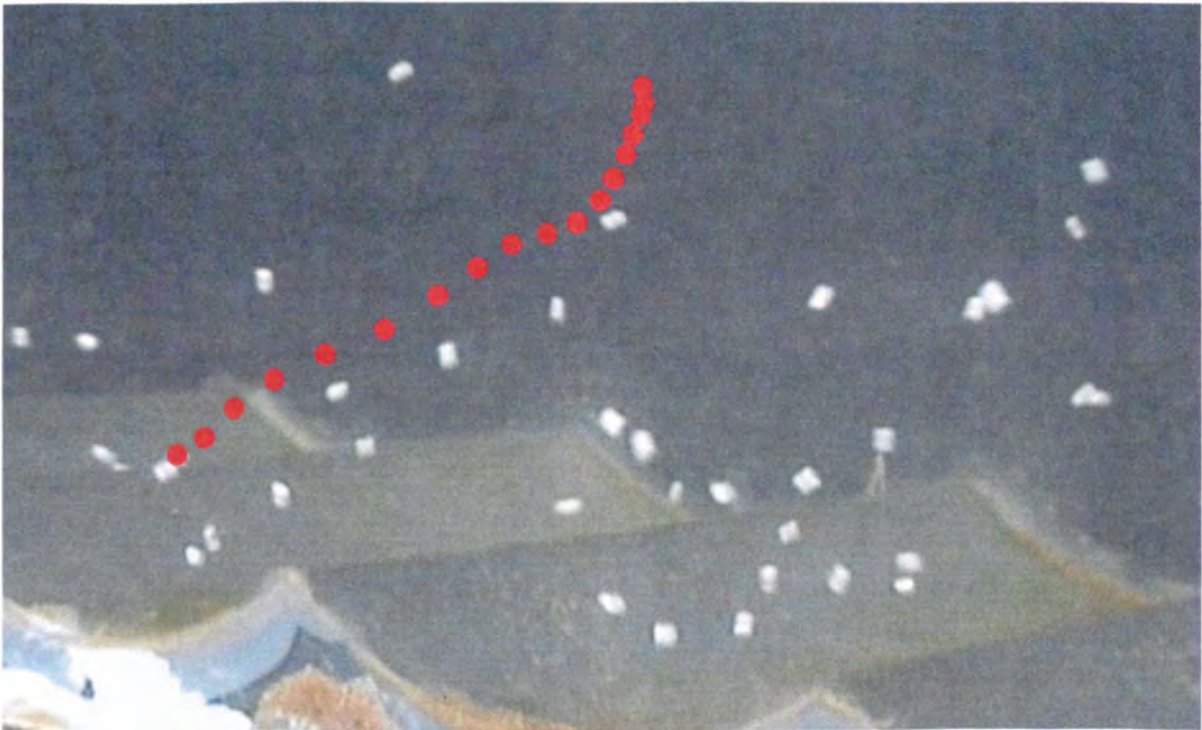
Figure 7.10: Composed picture of the movement of a single particle under waves. The wave height, wavelength and water depth were about 8 cm, 75 cm and 45 cm, respectively. Two stages of movement can be identified. The first one with horizontal and vertical movement and the second one with predominately vertical movement.
