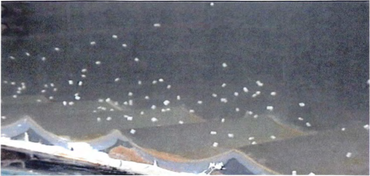
Figure 7.9: Suspension of plastic particles under wave motion. The wave height, wavelength and water depth were about 8 cm, 75 cm and 45 cm, respectively.
