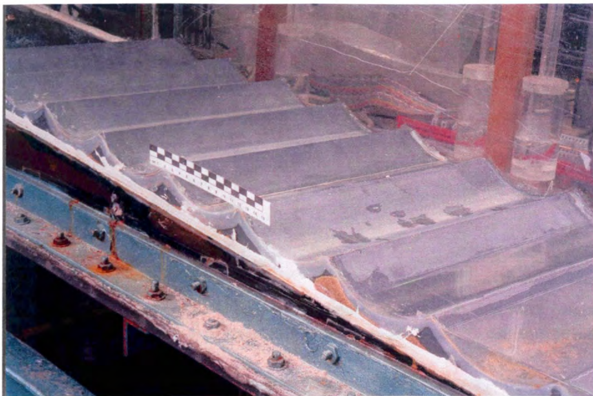
Figure 7.7: Plastic rippled bed in the laboratory wave flume. The ripple height is 2 cm and the wavelength is 10 cm.
