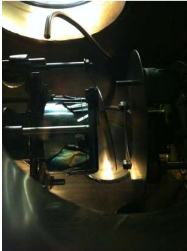
Fig. 3.4 Inside Chamber #2: the gas inlet opening on top of the heater and the shutter covering the substrate
