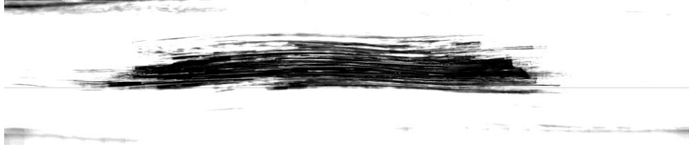
Figure 20 20x macro-image of the impregnation developed on bottom face of the tow. This image represents a collage of 300 micrographs.
