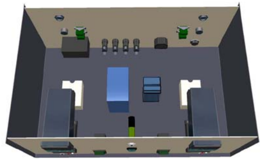
Figure 11.9 CAD drawing of the layout of the rear components inside the control box
