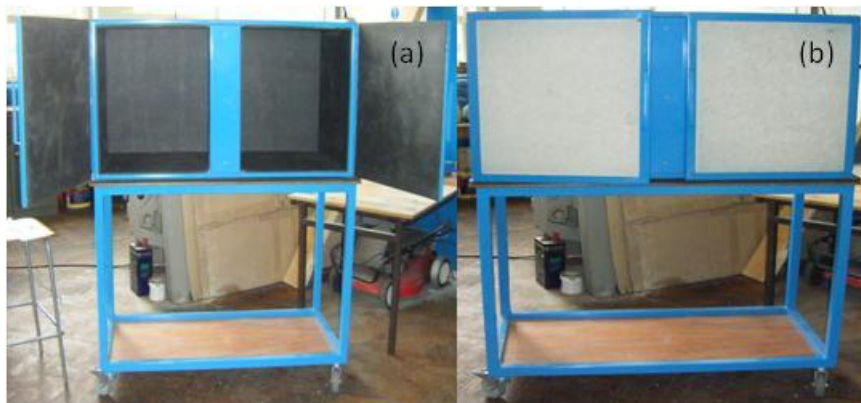
Figure 3.4: Sound resistant rig with (a) doors open and (b) doors closed.
