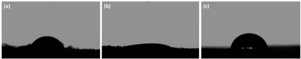
Figure 5.6 Images of a drop of water soaking into the surfaces of (a) cotton, (b) denim and (c) silk, produced by a goniometer. Frame is taken from a video at 0.6 seconds.
