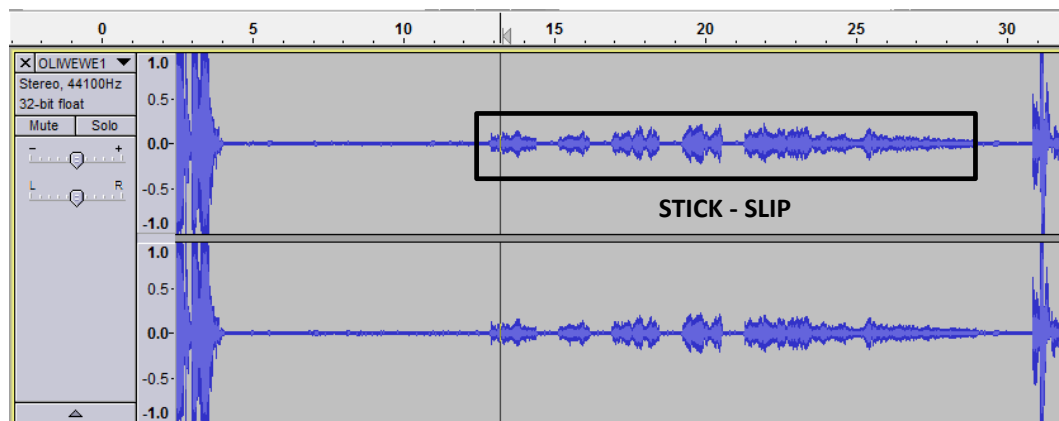
Figure 3.9 A visual example of all stages of noise produced from experimental methodology seen from left to right; doors of the SRR closing, background noise from laboratory, SDS noise, fabric noise, background noise and doors opening of the SRR.
