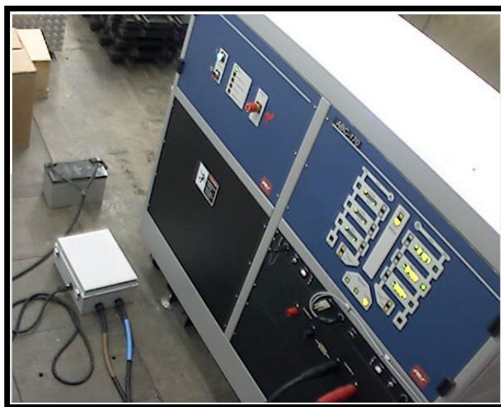
Figure 19 Structure of connection between battery and battery cycler
