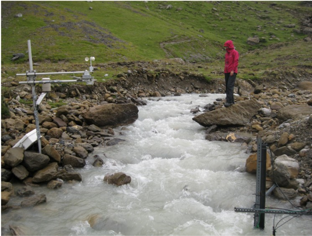
Plate 2.4. Taillon stream (1850m a.s.l.) roughly 100m above the confluence with the Tourettes stream, July 2011. The automatic weather station (left) and river flow gauging station (right) are in the foreground.
