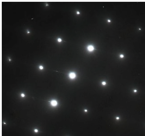
Figure 4.1.5 (a) TEM microstructure of AR sample and corresponding SAD patterns of (b) M_{23}C_6 carbide ( B=[\bar{1}12] ) from B area and (c) \alpha -FCC phase ( B=[1\bar{1}0] ) from C area.
