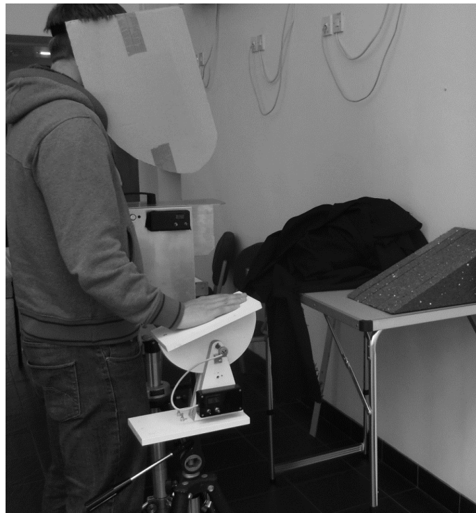
Figure 2.5. A photograph of the set-up used in experiment 2. The participant is shown wearing a novel device that hides their hand from view while making palm-board judgements without restricting their arm or wrist movement.
