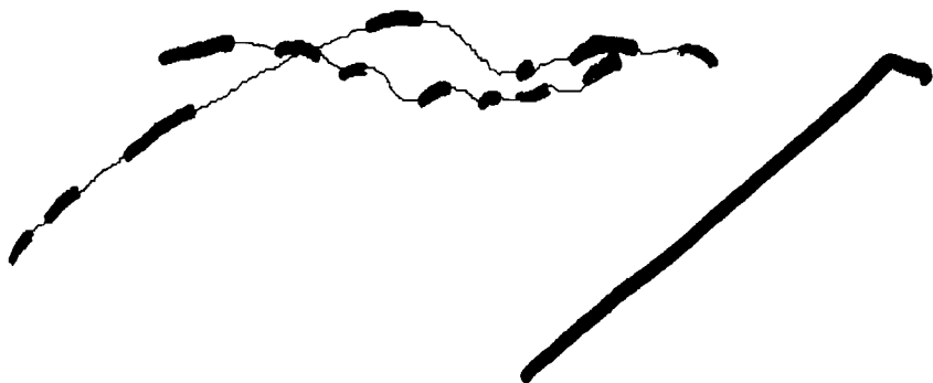
Figure 4. The cycloid-like trajectories of two particles entrained into the shear layer and transported downstream. The crest velocity is about 0.36m/s. The bedform angle is 30 degrees to the horizontal but appears larger due to graphical manipulation.
