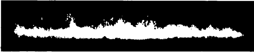
Figure 14. Grass (1974). Sand suspended by ejection events in a flat plate turbulent boundary layer. The sand visualises the coherent flow structures.
