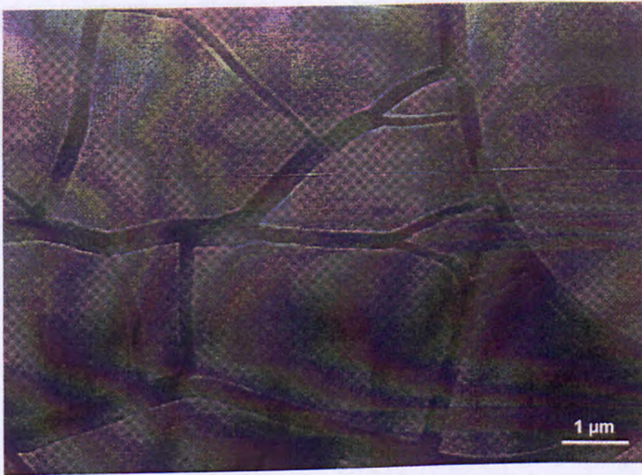
Figure 2.20: SEM micrograph of 53 nm thick \text{SiO}_x biaxial fragment morphology at saturation 129 .
