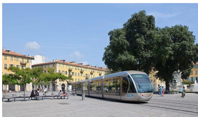
Operation With Energy Provided by the Batteries (Charles Watson, 2009)
