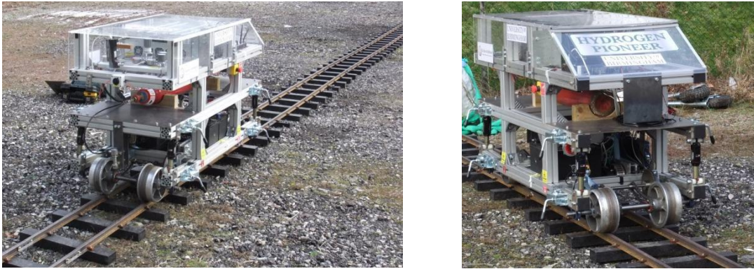
Figure 71: Hydrogen Pioneer on Test Track Ready for Vehicle Efficiency Evaluation Tests (Author's Collection, 2013)
