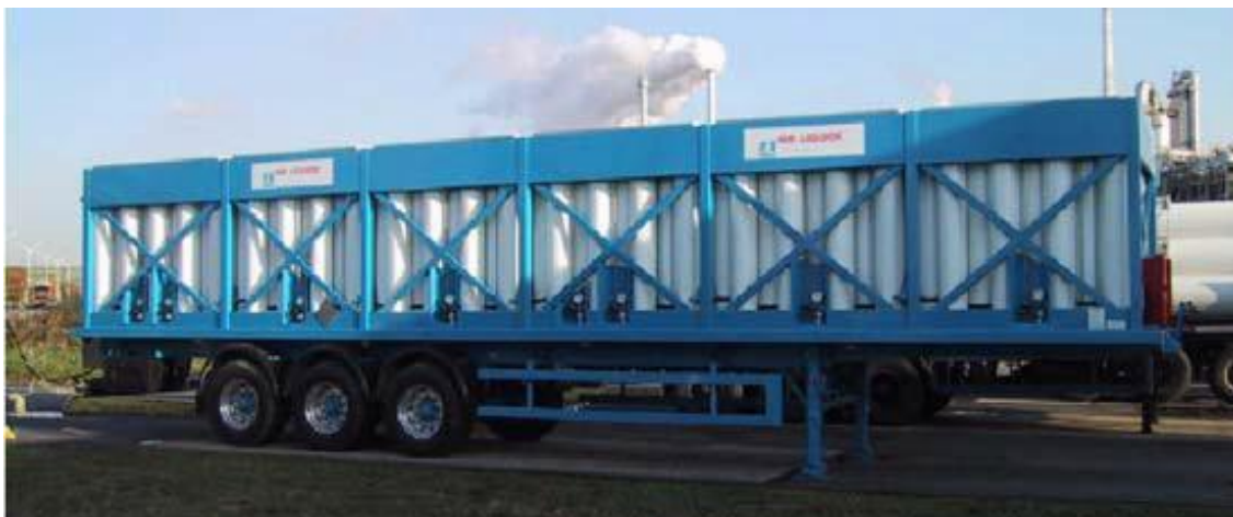
Figure 35: Trailer With Compressed Gas Hydrogen Cylinders in Bundles (Perrin, 2007)
