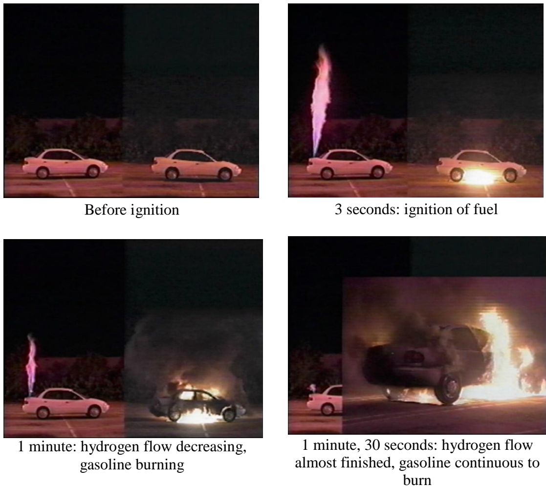
Figure 18: Video Frames of Fuel Leak Experiment at the University of Miami The Hydrogen-Powered Vehicle on the Left, Gasoline-Powered Car on the Right (Swain, 2001)
