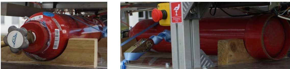
Figure 34: 200 bar Compressed Hydrogen Cylinder Installed in a Hydrogen Locomotive Courtesy and Copyright Jonathan Tutchter, 2012
