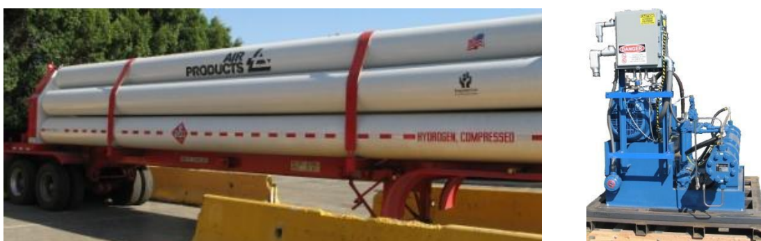
Figure 23: 200 bar Hydrogen Tube Trail and Compressor-Pump (Author's Collection, 2009)
