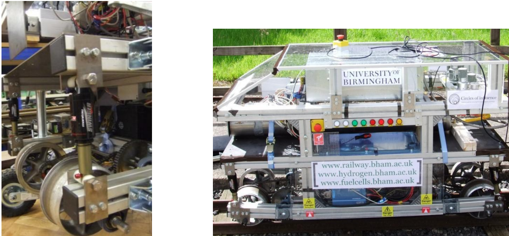
Figure 51: Air Suspension of the Hydrogen Pioneer (Author's Collection, 2012)
