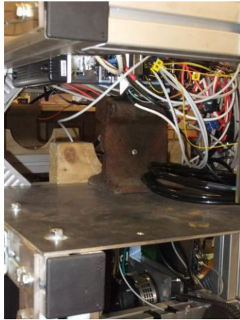
Figure 67: Additional Weights on the Locomotive to Account for the Mass of a Hydrogen Tank (Author's Collection, 2013)
