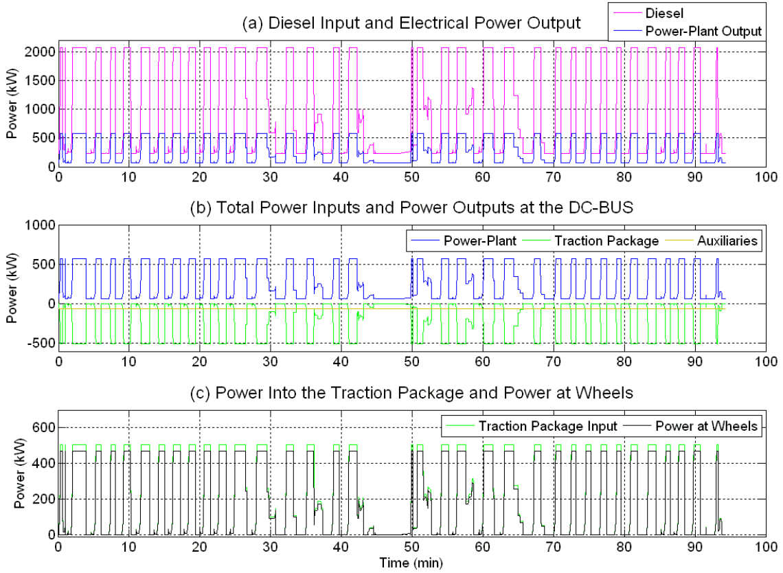
Figure 105: Power Across the GTW Drive-System
