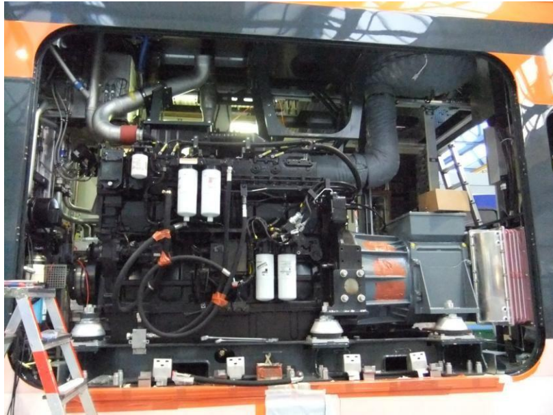
Figure 109: Diesel-Generator Set in a FLIRT Power-Module (Author's Collection, 2013)
