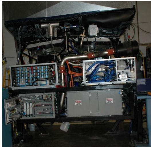
Figure 111: Vehicle Projects' Fuel Cell System Including Ancillaries Under Test in Denver (Miller, et al., 2009)
