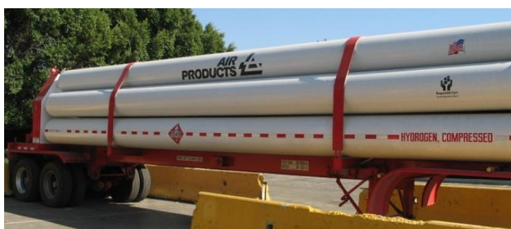
Figure 33: Hydrogen Distribution in a 200 bar Tube Trailer (Author's Collection, 2009)
