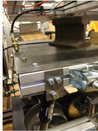
Figure 67: Additional Weights on the Locomotive to Account for the Mass of a Hydrogen Tank (Author's Collection, 2013)
