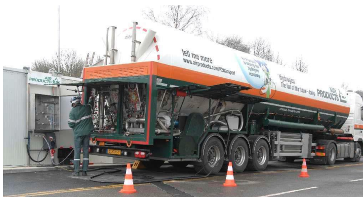
Figure 36: Dual-Phase Tanker Delivering Hydrogen Gas to a Filling Station (Williamson, 2011)
