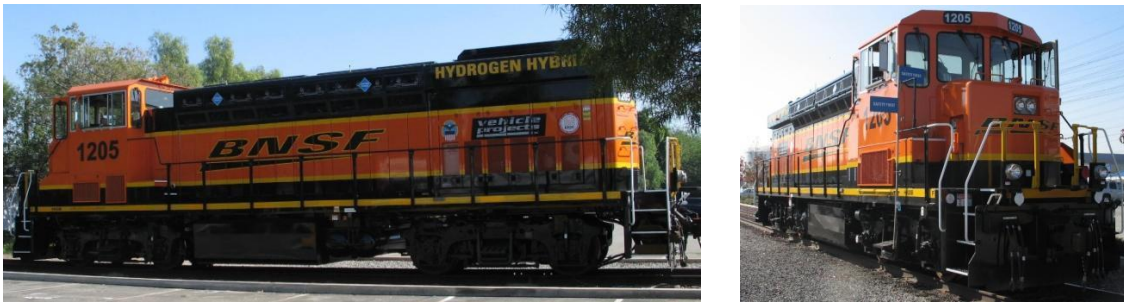
Figure 21: Vehicle Projects' Hydrogen-Hybrid Switcher Locomotive (Author's Collection, 2009)
