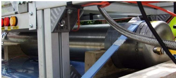
Figure 59: Metal-Hydride Hydrogen Storage Tank (Author's Collection, 2012)
