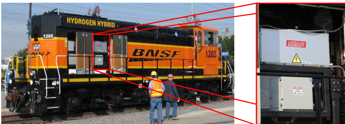
Figure 112: Illustration of a Fuel Cell Stack in Vehicle Projects' Hydrogen-Hybrid Switcher (Author's Collection, 2009)
