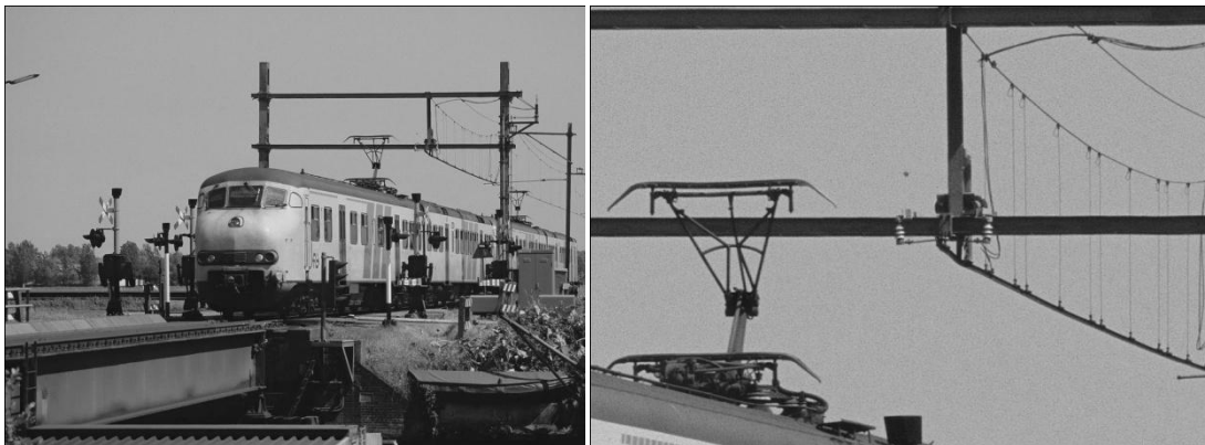
Figure 2: 75 m Gap in Overhead Electrification Infrastructure at Alphen aan den Rijn in the Netherlands 1
