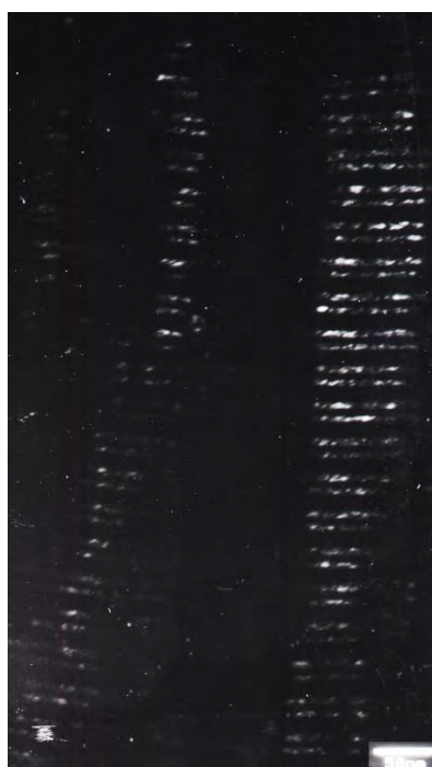
Figure 4.2.5- 6 Dark field images of Sublayer II of C-I-10, showing the CrN-like fcc-MeN phase
