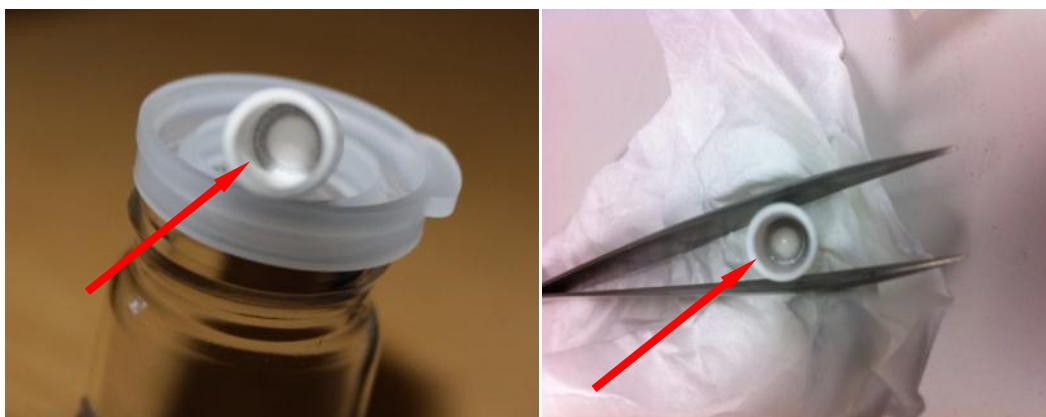
Fig. 4.12 Image of TGA crucibles after heating the \text{Li}^+ -BIRM-1 to 900\text{ }^{\circ}\text{C} , illustrating the solid residue thin layer melted on the internal layer of the crucibles.
