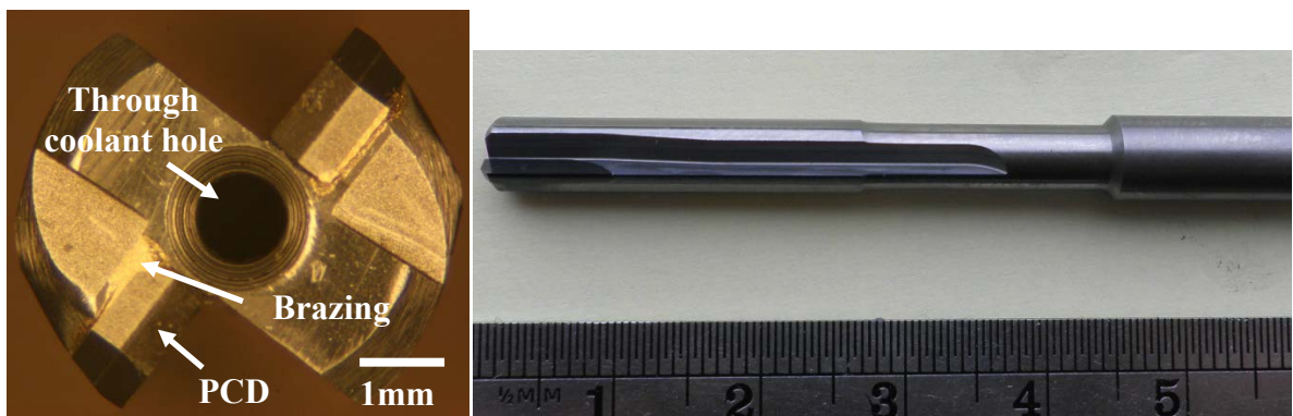
Figure 61: Mapal brazed Syndite CTB002 PCD reamer
