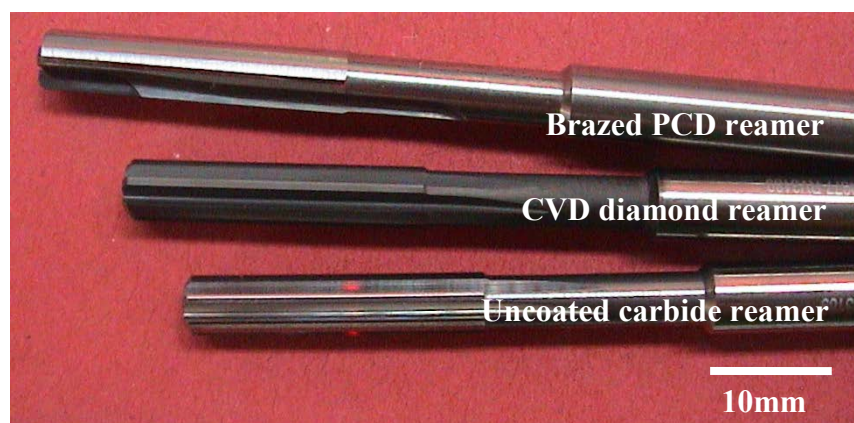
Figure 68: Uncoated, CVD diamond coated carbide and brazed PCD reamers
