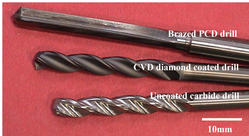
Figure 65: Uncoated, CVD diamond coated carbide and PCD drills
