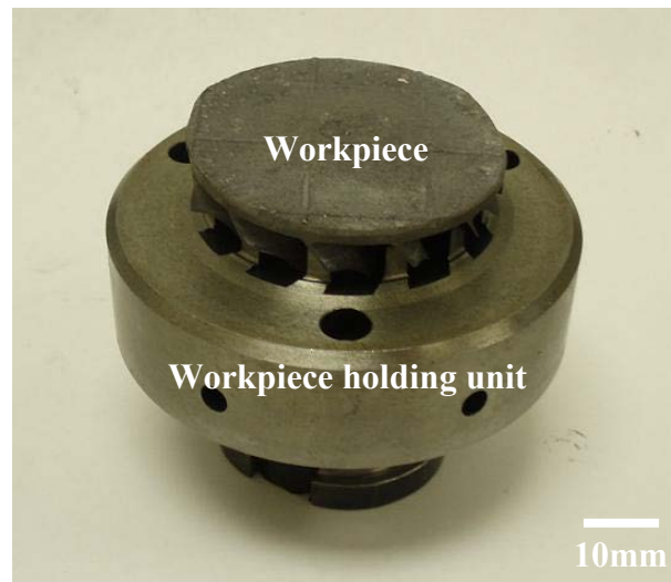
Figure 70: Workpiece and work holding unit used in Sterling
