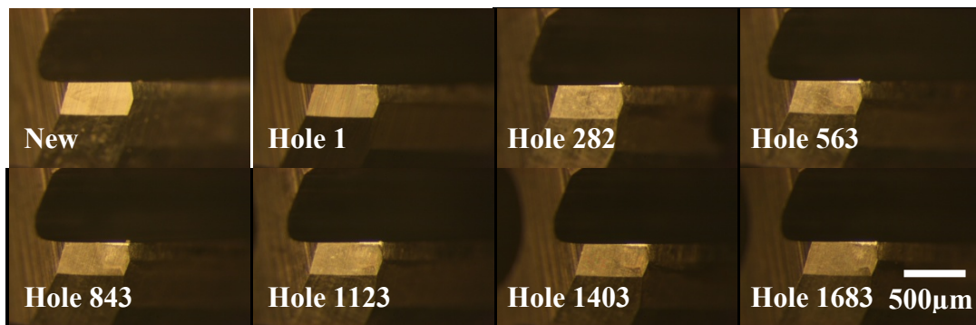
Figure F2: Tool wear micrographs of uncoated carbide reamer under 70bar through-hole cutting fluid, 96m/min cutting speed (Test 2)
