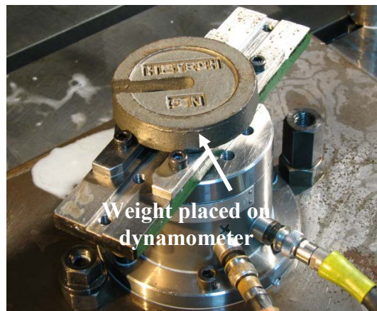
Figure 76: Typical force calibration on the dynamometer
