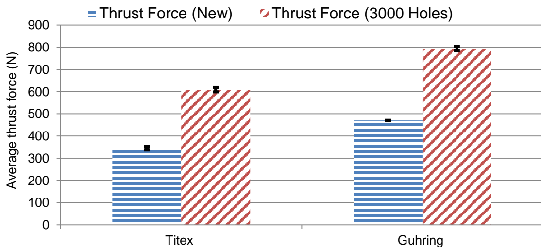
Figure 105: Average maximum drilling thrust force by Titex and Guhring drills
