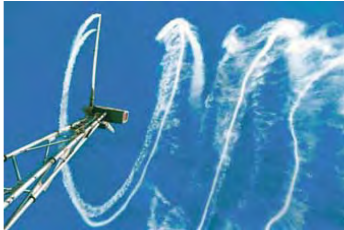
Figure 3-3 Wake effect demonstration (Source: Riso National Laboratory, Denmark)
