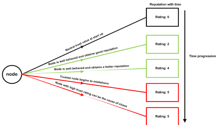
Figure 2.2: Node behaves as expected for some time to build a good reputation and suddenly begins to misbehave, such that the reputation fails to detect the node
