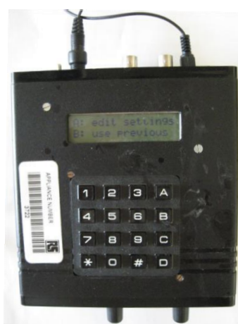
Figure 6.3: Picture of the control box of the flow-through microdispenser.
