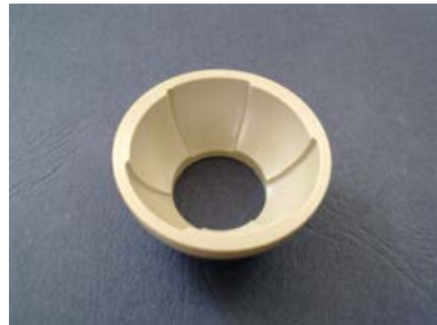
(d) PEEK cup which holds the SmCo sphere within the NdFeB shell
