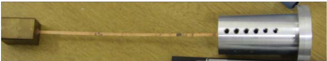
Figure 2.3: Image of torsion strip before installation into the apparatus.
