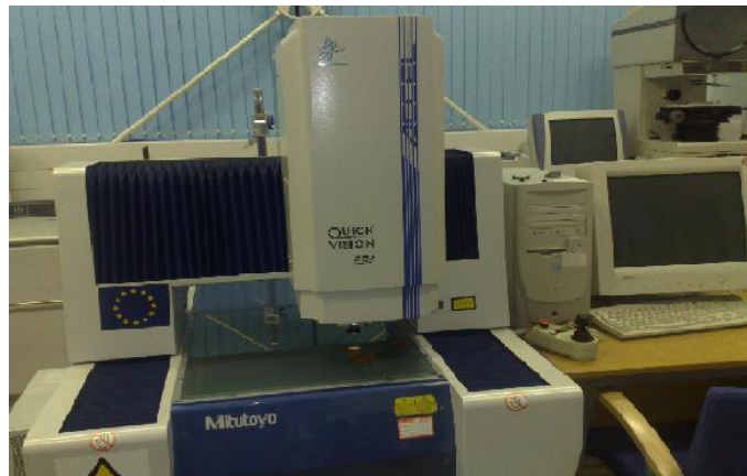
Fig. 4.6 a: QuickVision® Coordinate Measuring Machine (CMM)
