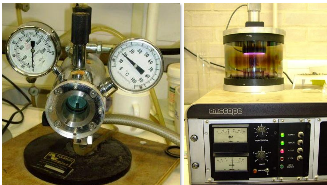
Figure 3.7.A. Critical point drier of carbon dioxide and 3.7.B sputtering system of platinum.
