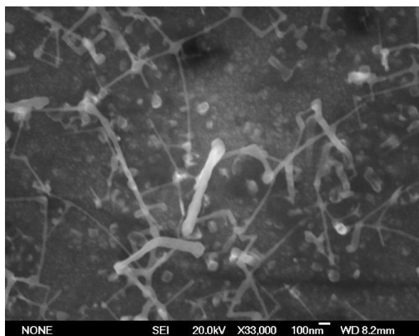
SEM 1.8 Nanorod diameters <100 nm with some networks.
