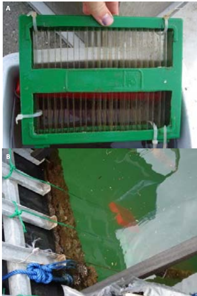
Figure 2.8. A) Holder containing ~30 glass slides (76x26x1mm) (Section 2.7.5.1). Each glass slide was separated from the following one by ~ 1 cm. B) Holders containing the slides were submerged at about 1 m depth for 3-d to allow biofilm colonization. After 3-d biofilms were transported to the laboratory.
