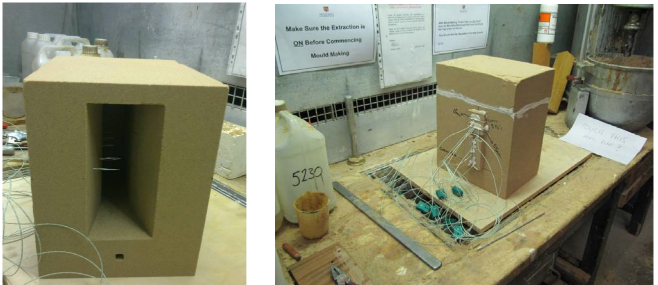
Figure 20: Images showing the thermocouple locations in the castings and how they held in position
