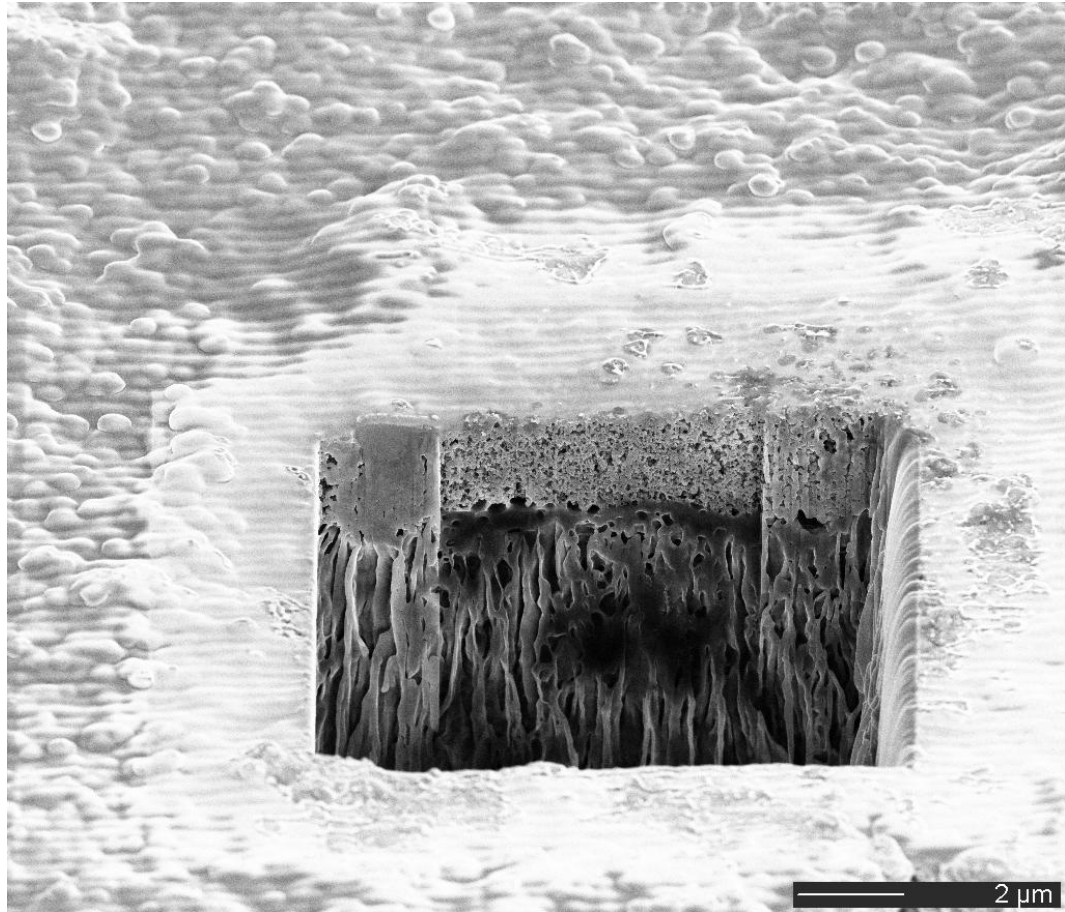
Figure 6.14. Low magnification SEM image of the trench side wall polished through low current 30 pA ion beam, Pt deposited area and milled.
