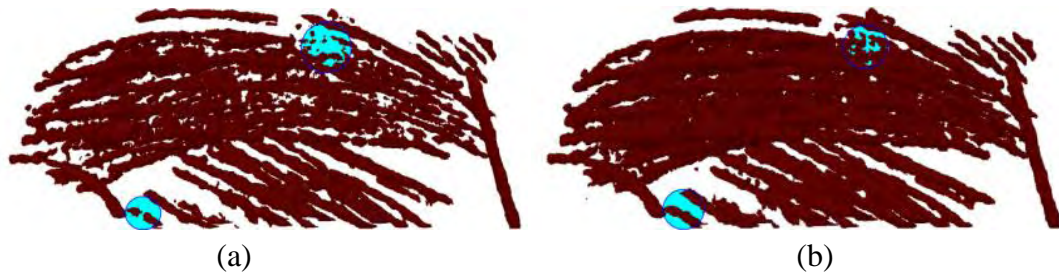
Figure 3.14. Threshold variation as small as 5% makes a significant effect on fibre's continuity. The blue circles are examples of discontinuity; a) low threshold based on Otsu's method and; b) is high threshold.
