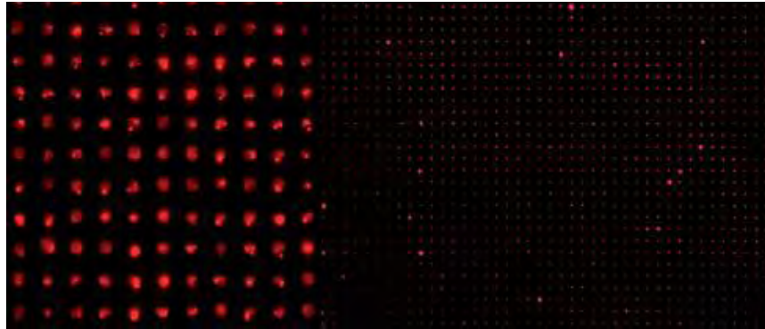
Fig 1.17 Arrays of RFP E. coli directly patterned onto porous aluminium oxide using PDMS pins controlled with a micromanipulator 143
