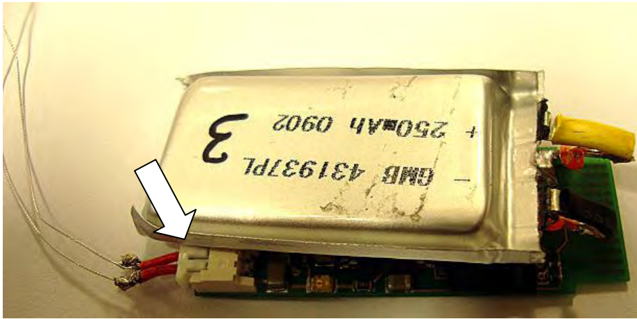
Image demonstrating where the male receptacle housing is to be inserted (white arrow)
