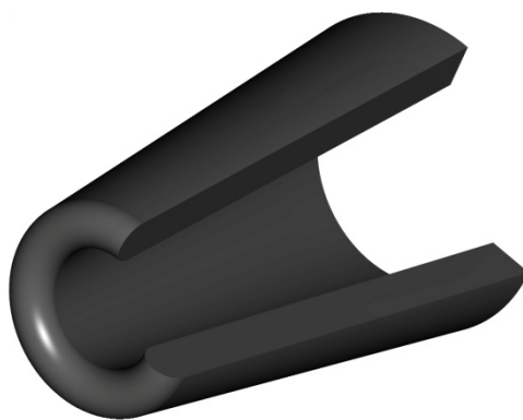
Figure 6.19 A schematic of a micropipette tip. If the tip is formed in a fluid phase then the tip should have a semispherical shape.
